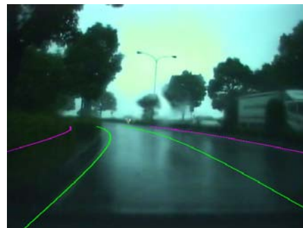
Fig. 1: The result of road geometry estimation projected on real scene without visual detection in stormy weather
